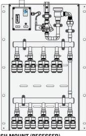
FLUSH MOUNT (RECESSED) WITH PUSH-IN CONNECTIONS (CTS) ELECTRONIC TRAP PRIMERS Model No. 272FM-CTS Series
