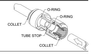
Pull on the fitted Tubing to ensure it is secure. Tube should not come free from the Fitting. Water test the Connection assembly prior to leaving the site to ensure there are no leaks.
