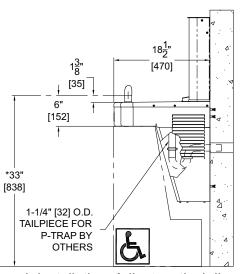
**NOTES:** Dimensions indicated (\*) are for ADA frontal approach installation. Adjust vertical dimension (\*) as required to comply with federal, state, and local codes. For Child ADA compliant parallel approach, decrease Bubbler spout height to 30" maximum above finished floor. Provide clear floor space as required.
