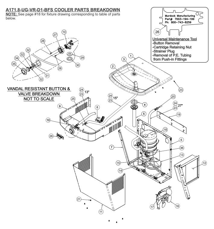
Standard A171.8-UG-VR-BFxS series refrigerated ADA cooler shown. All 1/4" O.D. Plastic tubing (23) must be insulated with (24) foam insulation.
